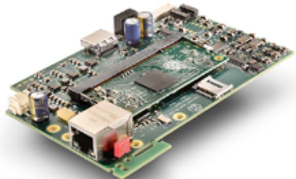
The N31 Roon input module board
